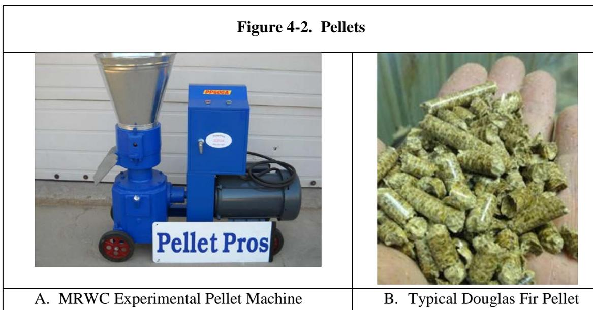
While MRWC samples were relatively dry (<8%-10% MC)<sup>19</sup>, wood for making pellets must be uniformly less than 8% MC. A dryer would be required to make a fuel product like the pellets shown in Figure 4-2B. Commercial pellet production would require a dryer that is typically sized for 1-6 dry tons per hour.
